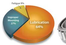
Sixty-four percent of bearing failures are lubrication related. Less than 9% of bearings reach their L10 design life expectancy. Source: American Bearing Manufacturers Association (ABMA)
