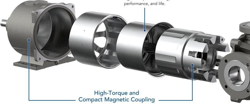
High-strength magnetic couplings come standard to allow more operational flexibility for tough applications and potential system-upset conditions. The patented rotor magnet assembly mounts directly to the rotor for an extremely compact design. High-temperature, greased-for-life bearings support the outer magnet assembly.
